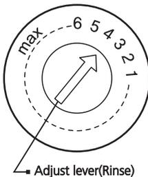
The rinse aid reservoir has six settings. Both the recommended setting and the factory setting is "4". If the dishes are not drying properly or are spotted, adjust the dial to the next higher number until your dishes are spot-free. Reduce it if there are sticky whitish stains on your dishes or a bluish film on glassware or knife blades.
