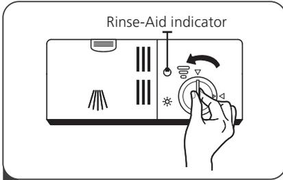
**1** To open the dispenser, turn the cap to the "open" (left) arrow and lift it out.
